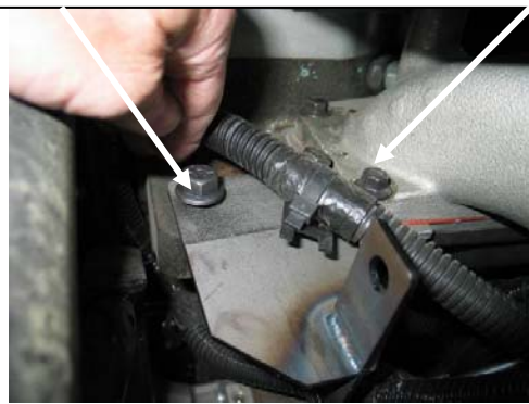
Photo #2 - Here is the photo of the metal bracket mounted – use existing bolt on truck & additional one is included in kit to self tap in the empty
